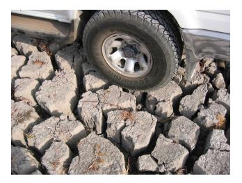
amount of clay that they contain. Geotechnical professionals usually classify soils as having very low, low, medium, high or very high expansion or swell potential according to guidelines in building codes. There are specific laboratory tests to evaluate a soil's expansion potential.
